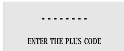
Enter the VCR PLUS+ code (three-to-eight digit number) of the show you wish to record using the 10-key pad on the remote control. The following screen will appear:
