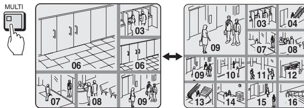
**Note:** The DSR-3709 can display in the plus mode, but it cannot switch split-screens.
