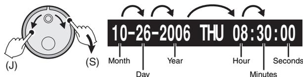
When the setting of "Minutes" is complete, the cursor moves to <DAYLIGHT SAVING>, and the clock starts from 00 seconds.
