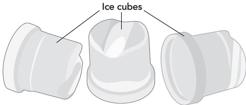
Normal cubes are tapered cylinders. If the cubes are ragged and misshaped, mineral scale must be removed from the ice making system.
