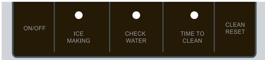
3. Press and HOLD the both the Clean-Reset and On/Off buttons for 5 seconds. The Time to Clean light will blink on and off.
