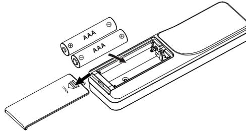
Install two “AAA” batteries in the compartment according to the polarity markings inside the compartment as shown in the illustration. If the batteries are installed incorrectly the remote control will not work. After installing the batteries replace the battery compartment cover.
