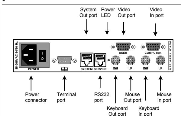
Connect a keyboard, monitor, mouse plus the 3 in 1 CPU cable and Power cord to the UPM and computer as illustrated in the figure below. Connect the Power cord. Only use the power cord supplied with the UPM.
