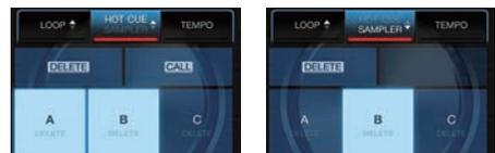
The hot cue or sampler mode can be selected by tapping [HOT CUE/SAMPLER].
