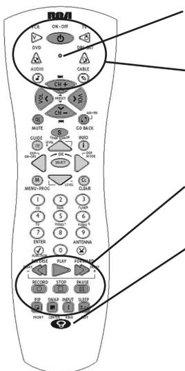
**Indicator Light**—flashes when a valid key is pressed to indicate the remote is working. Status of this light is important when you are programming the remote.
