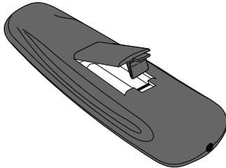
1. Remove the battery compartment cover.
