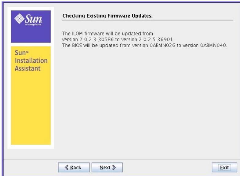
Follow the on-screen instructions until the upgrade has completed. Upgraded code will not be used by the system until after a reboot.
