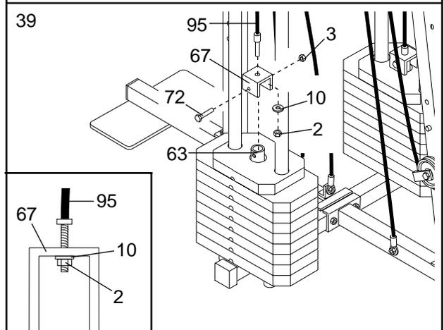
Attach the Small "U" Bracket (67) to the indicated Weight Tube (63) with a 5/16" x 1 3/4" Bolt (72) and a 5/16" Nylon Locknut (3).
