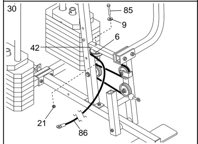
31. Wrap the Low Cable (86) around a 3 1/2" Pulley (15). Attach the Pulley and a Cable Trap (66) to the Press Frame (17) with a 3/8" x 3 1/2" Bolt (16), a 3/8" Washer (9), and a 3/8" Nylon Locknut (21). **Be sure that the Cable Trap is turned to hold the Cable in place and that the Cable is routed around the Pulley as shown.**
