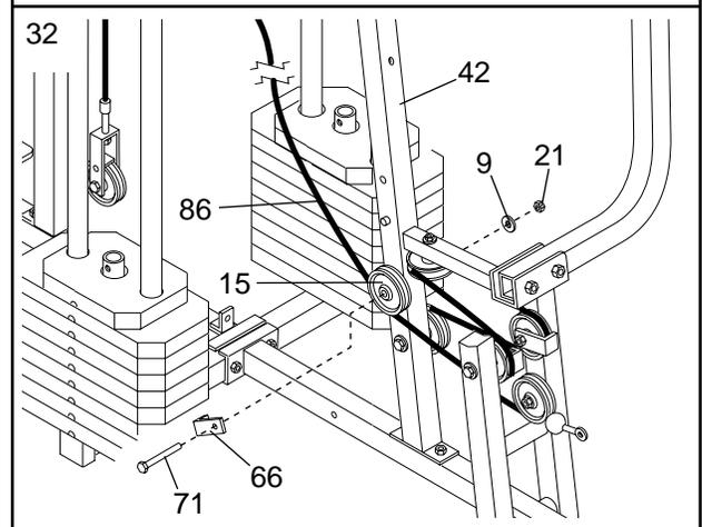
33. Route the Low Cable (86) over the lower 3 1/2" Pulley (15) attached to the "I"-Plates (81). The Cable must be routed from the direction shown.
