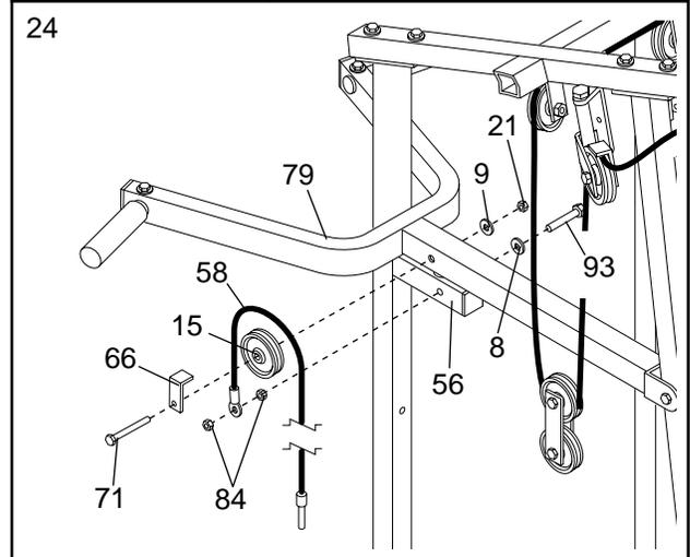
Wrap the Press Cable (58) around a 3 1/2" Pulley (15). Attach the Pulley and a Cable Trap (66) to the Squat Arm (79) with a 3/8" x 3 3/4" Bolt (71), a 3/8" Washer (9), and a 3/8" Nylon Locknut (21). **The Cable Trap must be turned to hold the Cable in place.**
