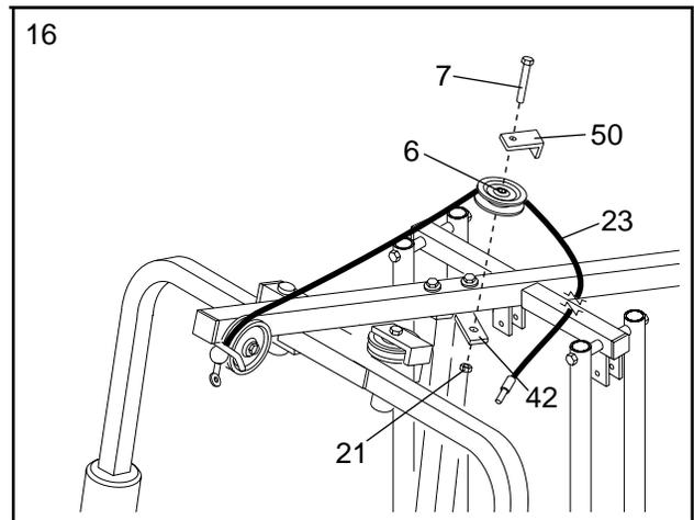
17. Route the High Cable (23) around the “V”-Pulley (6) on the Left Arm (47). **Be sure that the Cable is in the groove of the Pulley and that the Long Cable Trap (50) is positioned to hold the Cable in place.** Tighten the 3/8” x 2 1/2” Bolt (7) and the 3/8” Nylon Locknut (not shown).
