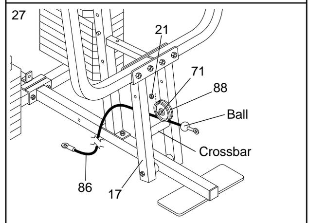
**Note: You may need to remove the 3 1/2" Low Pulley (88) from the 3/8" x 3 3/4" Bolt (71) to properly route the Low Cable (86).**
