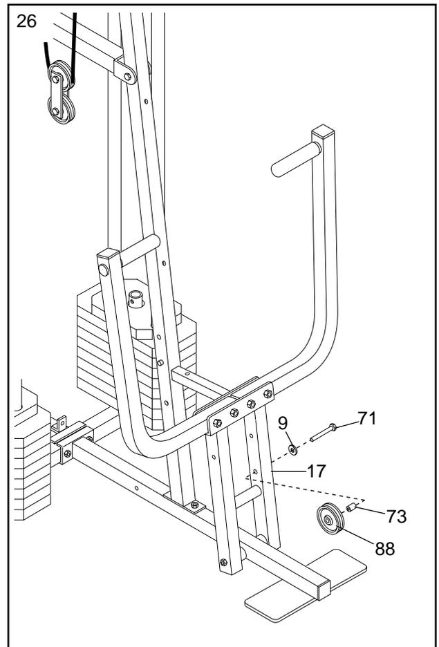
27. **Locate the Low Cable (86).** Slide the Low Cable into place under the 3 1/2" Low Pulley (88). **Be sure that the end of the Cable with the ball is on the indicated side of the Press Frame (17) and that the Cable is between the Pulley and the crossbar on the Press Frame.** Fully tighten a 3/8" Nylon Locknut (21) onto the 3/8" x 3 3/4" Bolt (71).
