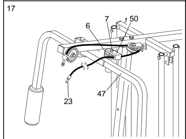
18. Route the High Cable (23) around the “V”-Pulley (6) on the Right Arm (48). **Be sure that the Cable is in the groove of the “V”-Pulley and that the Long Cable Trap (50) is turned to hold the Cable in place.** Tighten the 3/8” x 2 1/2” Bolt (7) and the 3/8” Nylon Locknut (not shown).
