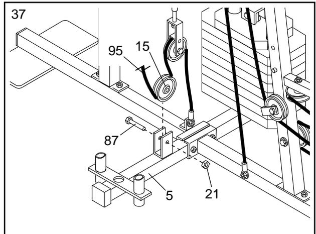
38. Wrap the Rear Cable (95) around a 3 1/2" Pulley (15). Attach the Pulley to the indicated bracket on the Top Frame (55) with a 3/8" x 1 3/4" Bolt (87) and a 3/8" Nylon Locknut (21). **The Cable must be routed from the direction shown.**
