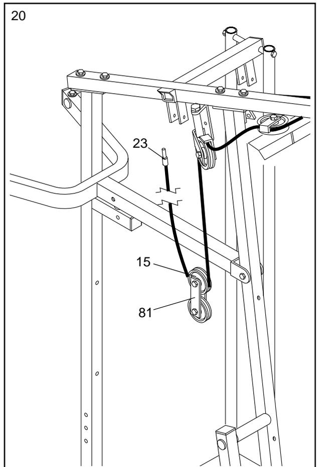
21. Wrap the High Cable (23) around a 3 1/2" Pulley (15). Attach the Pulley to the Top Frame (55) with a 3/8" x 1 3/4" Bolt (87) and a 3/8" Nylon Locknut (21).
