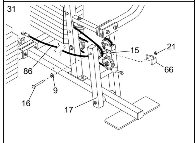
32. Wrap the Low Cable (86) around a 3 1/2" Pulley (15). Attach the Pulley and a Cable Trap (66) to the indicated hole in the Front Upright (42) with a 3/8" x 3 3/4" Bolt (71), a 3/8" Washer (9), and a 3/8" Nylon Locknut (21). **Be sure that the Cable Trap is turned to hold the Cable in place and that the Cable is routed around the Pulley as shown.**
