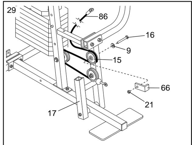
30. Wrap the Low Cable (86) around a "V"-Pulley (6). Attach the "V"-Pulley to the indicated hole in the Front Upright (42) with a 3/8" x 3 1/4" Bolt (85), a 3/8" Washer (9), and a 3/8" Nylon Locknut (21). **Be sure that the Cable is in the groove of the "V"-Pulley and that the Cable is routed around the "V"-Pulley as shown.**
