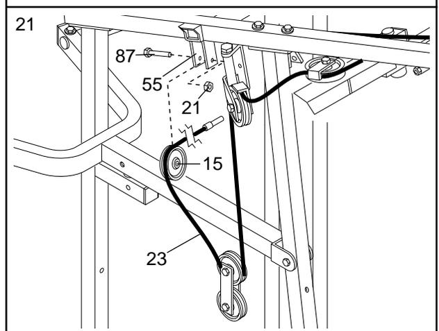
22. Wrap the High Cable (23) around a 3 1/2" Pulley (15). Attach the Pulley to the Top Frame (55) with a 3/8" x 1 3/4" Bolt (87) and a 3/8" Nylon Locknut (21).
