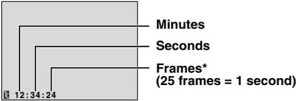
\* Frames are not displayed during recording. If recording starts from a blank portion, the time code begins counting from "00:00:00" (minute:second:frame). If recording starts from the end of a previously recorded scene, the time code continues from the last time code number.
