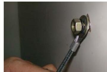
Fix the other end of the Safety Strap to one of the upper wall mounting holes on the back of the HDTV, using a washer under the screw head.
