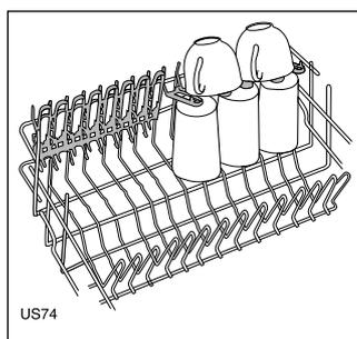
For glasses with long stems (according to the size and dimensions), set the glass holder to the left-hand or right-hand position.
