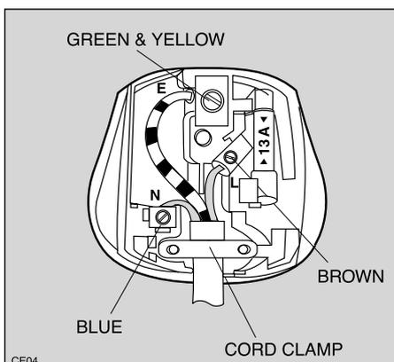
If you fit your own plug, the colours of the wires in the mains lead of your appliance may not correspond with the markings identifying the terminals in your plug.
