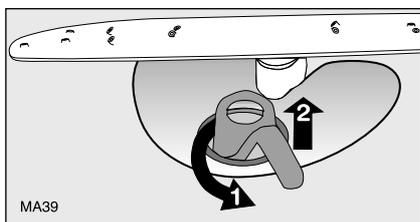
4. Take hold of the coarse filter (A) by the handle with the hole and remove from the microfilter (B).
