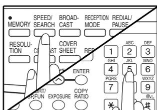
If it is not correct, press the [CLEAR] key (C) to backspace and clear two digit at a time, and then enter the correct number.
