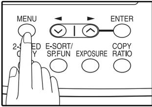
**2 Press the [◀] key (⓪) or [▶] key (Ⓜ) until "2:ENTRY MODE" appears, and then press the [ENTER] key.**
