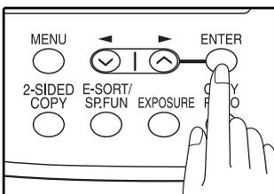
**4 Press the [◀] key (▽) or [▶] key (△) to scroll through the names. Stop when the desired name appears in the display.**
