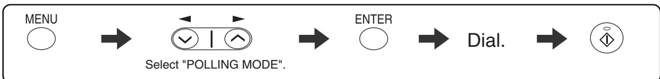
\* Another fax machine can also call your fax machine and request automatic transmission of a original placed in your machine. For this to take place, the reception mode of your machine must be set to "AUTO".
