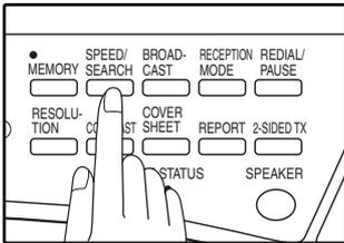
**2 Enter the first letter of the stored name by pressing the appropriate numeric key (the key below the marked letter) until the letter appears in the display.**
