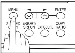
**2** Press the [◀] key (⏪) or [▶] key (⏩) until "2:ENTRY MODE" appears, and then press the [ENTER] key.
