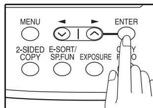
**3 Press the [◀] key (v) or [▶] key (^) until "2:DATE&TIME SET" appears, and then press the [ENTER] key.**
