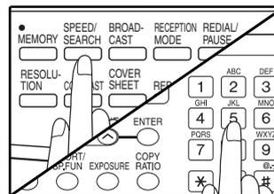
Dialing with a Speed Dial number and then press the [ENTER] key or [START] key (Ⓢ).
