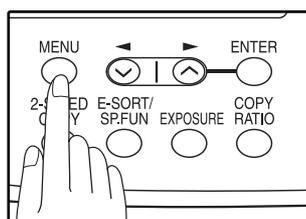
Press the [MENU] key to exit. If the number is a Rapid key number, you can write the name on the label above the appropriate Rapid key.
