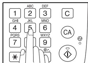
Enter your own fax number (maximum 20 digits) by pressing the Numeric keys. To insert a "+", press the [ \* ] key.
