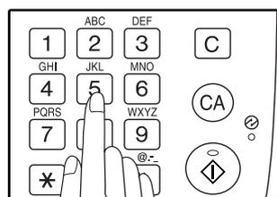
Enter your name by pressing the appropriate Numeric keys as shown on the left. Press each key repeatedly until the desired letter appears in the display (maximum of 40 characters).
