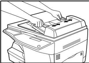
**3** Place the original face up and push it gently into the ADF/RADF. The top edge of the original should enter the fax first.
