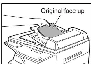
For the size and weight of two-sided originals that can be scanned using the RADF, see page 50.
