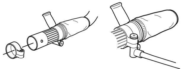
Assemble the intermediate pipe.
