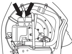
Pull out the spark arrestor screen and clean using a wire brush. Replace the spark arrestor screen if it is defective.
