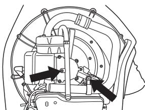
Loosen the muffler's 2 screws and remove the muffler.
