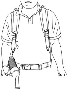
Tighten the side straps so that the pressure is evenly distributed across the shoulders.
