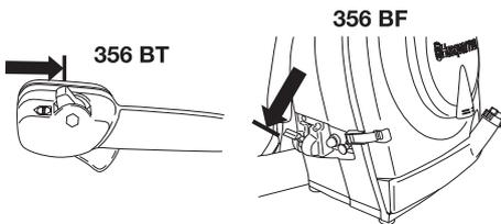
It is not allowed to set the stop switch in full throttle position.
