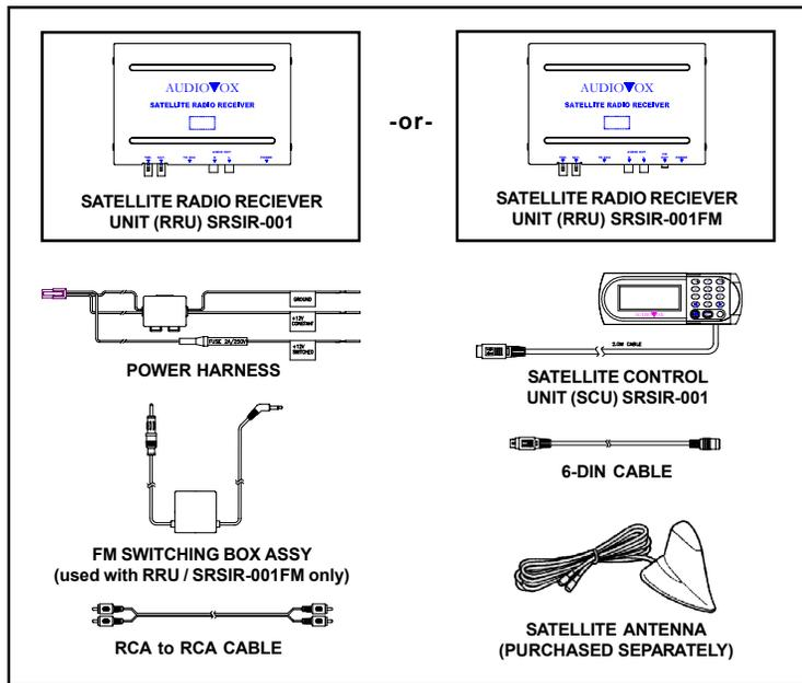
Figure 1. SIRIUS® Satellite Receiver System
