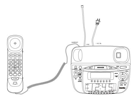
Push the modular plugs all the way into the sockets until a click is heard and the plugs are locked in place.
