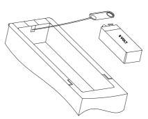
4.) Push the battery back into the battery compartment and replace the battery door. Turn the base unit right side up again.
