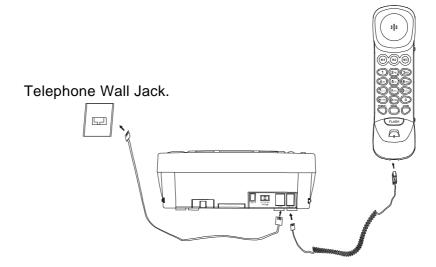
Push the modular plugs all the way in to the sockets until a 'click' is heard and the cords are locked in place.
