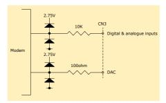
These I/Os are operated by AT commands in the modem.
