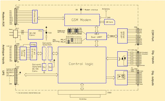
All models, except A-versions, has an onboard DC/DC converter that converts the incoming mains  $(+8-35V\ DC)$  to +5V. This power supply delivers +5V, up to 4A, to the module and to the PC/104 bus. A mains fuse F2 (1.6A) is placed on the rear side of the PCB, near KL1. In A-versions, where the DC/DC-converter is omitted, the module receives its power from the PC/104 bus.
