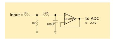
The analogue inputs are factory configured by choosing proper values for R1 and R2. In the table the values are shown for the different models. The input resistance is  $1M\Omega$  on all voltage input channels. The software interface is explained in section *PV-1800 register interface*.
