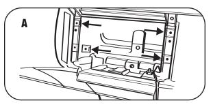
2 Remove mounting brackets "A" from the radio housing. (Figure B)
