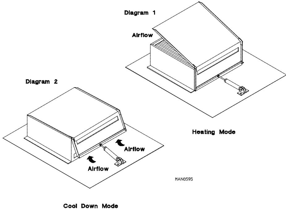
6. Steam Damper Air Piston (Flow Control) Operation Adjustment
