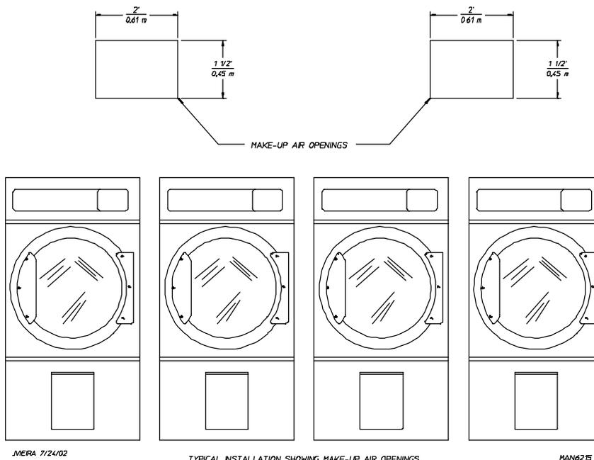
To compensate for the use of registers or louvers used over the openings, this make-up air **must be** increased by approximately thirty-three percent (33%). Make-up air openings **should not be** located in an area directly near where exhaust vents exit the building.
