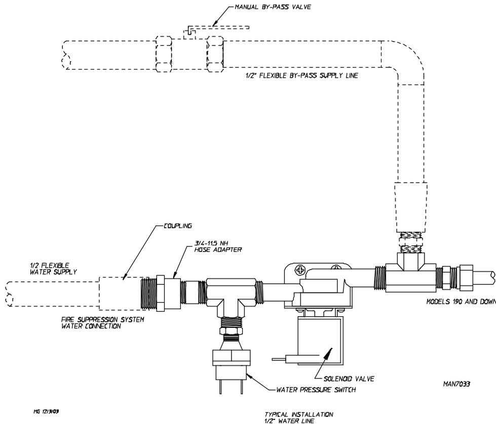
**WARNING:** If the water in the supply line or water solenoid valve freezes, the F.S.S. will be INOPERATIVE!!
