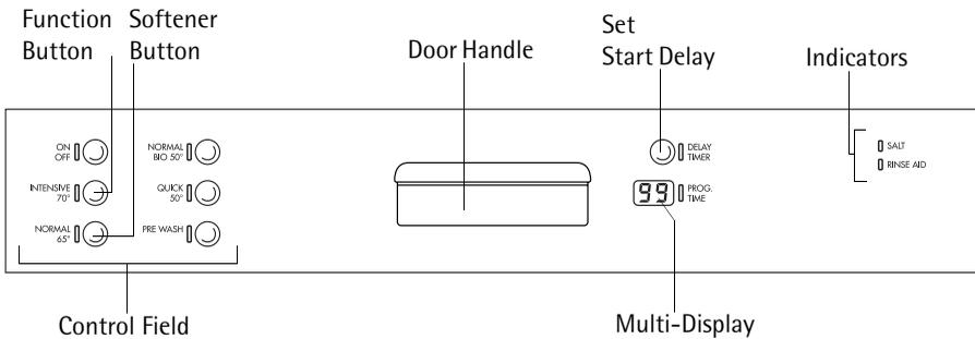
The **Control Field** comprises the ON/OFF switch and the programme buttons with LED indicators.
