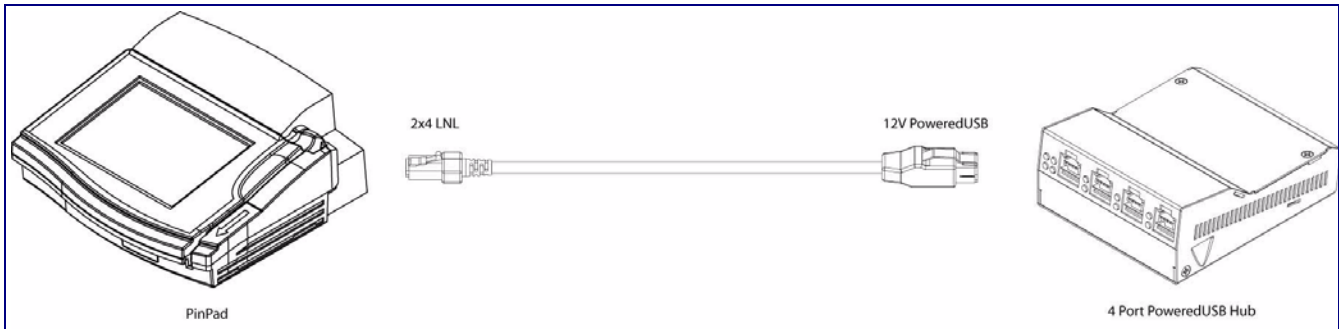
Figure 2-11. Cable, +12V PoweredUSB to 2x4 PoweredUSB
