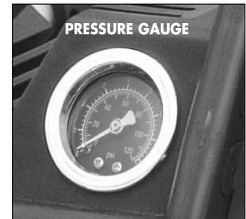
4. Monitor the pressure gauge. When desired pressure is reached, slide the Air Compressor/Inflator Switch to OFF; open thumb latch and remove connector from valve stem.
