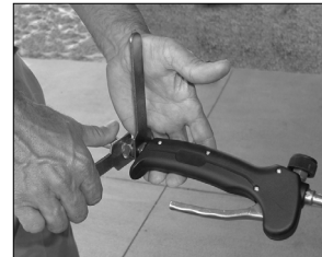
Figure 2 - Attaching gas line to handle (WT4500 shown, WT5500 similar)
