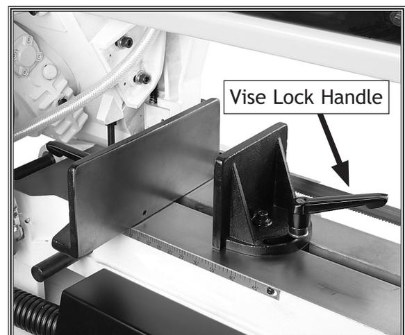
Figure 17. Front vise jaw lock handle.
