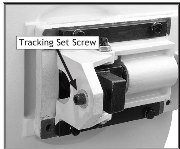
Figure 36. Tracking set screw.
