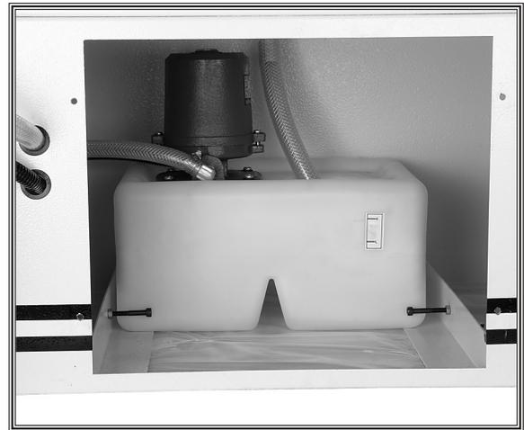
**Figure 24.** Coolant system reservoir and cover.
