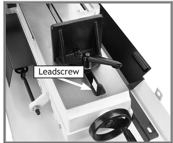
**Figure 28.** Vise leadscrew lubrication area.
