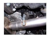
Install passenger side tailpipe/muffler assembly #C. Insert all welded nangers into rubber grommets. Secure tailpipe with clamp #D. Do not tighten.
