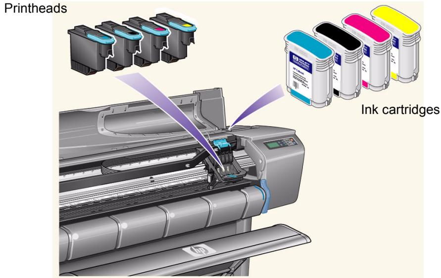
The Hewlett-Packard selection number on the ink cartridges and printheads makes it easy for you to find the correct HP ink supplies for your printer. Determine the color of the printhead or ink cartridge you need, then make sure you purchase or order the correct Hewlett-Packard printhead or ink cartridge. Each ink cartridge and printhead can be purchased separately from your usual Hewlett-Packard retailer. See [Ordering accessories](#).
