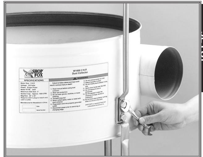
Figure 16. Installing upper bag support.
