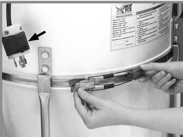
**Figure 3.** Unplug machine when emptying bags.
