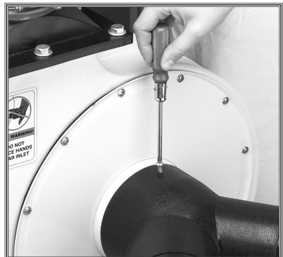
Figure 20. Securing inlet with screw.
