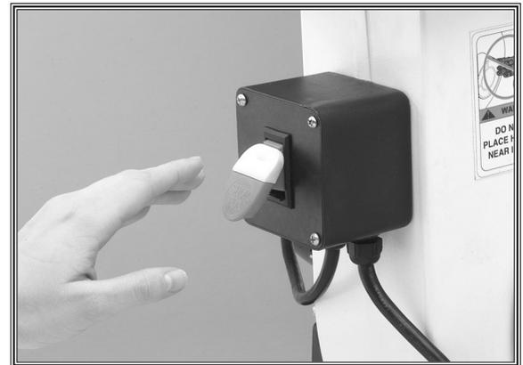
Figure 24. Hand position for emergency stop.
