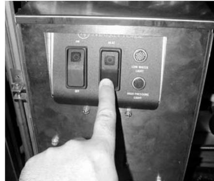
2. Energize heating circuit to pre-heat unit.
