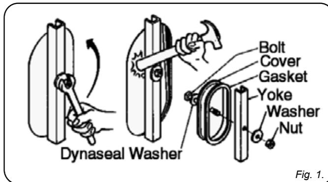
2. Remove the hand-hole cover as follows: (Refer to Fig. 1)
