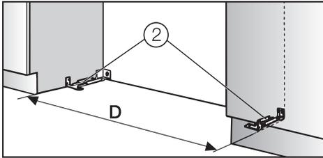
The distance "D" between the anti-tip brackets ② is the width of the appliance.
