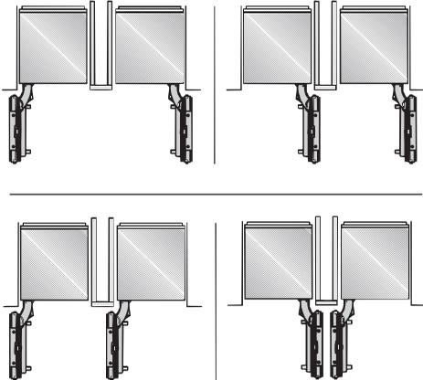
The minimum thickness of the partition is  $\frac{5}{8}$ " (16 mm).
