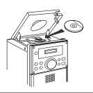
5 Close the CD compartment by firmly pushing the corner marked "PUSH CLOSE".
