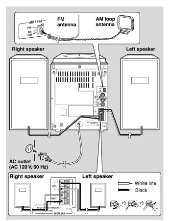
Make sure to unplug the AC power cord before any connections.
