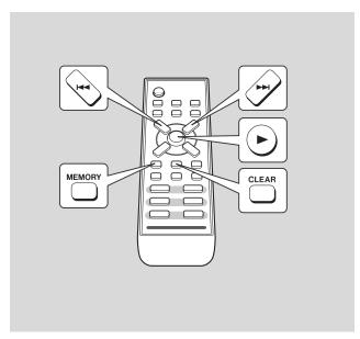
1 While in the stop mode, press the I◄◄ or ►►I button to select the desired track.
