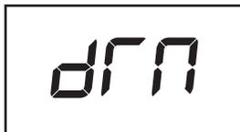
into the console. However, when you remove the key, the displays will remain lit, although the buttons will not function. If the demo mode is turned on, a “d” will appear in the left display while the information mode is selected. To turn on or turn off the demo mode, press the Speed decrease button.
