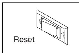
**IMPORTANT:** The console features a display demo mode, designed to be used if the treadmill is displayed in a store. If the displays light as soon as you plug in the power cord and press the power switch into the reset position, the demo mode is turned on. To turn off the demo mode, hold down the Stop button for a few seconds. If the displays remain lit, see THE INFORMATION MODE on page 14 to turn off the demo mode.
