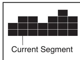
At the end of each segment, a series of tones will sound and the next segment of the profile will begin to flash. If a new speed and/or incline setting is programmed for the next segment, the speed and/or incline will appear in the display and the treadmill will automatically adjust to the new speed and incline settings.
