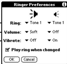
**Tip:** You can use both a ring tone and vibrate alert or use them separately. For example, you can set one position to ring softly and vibrate, and the other position to vibrate only. To preview a new sound, select Play ring when changed.
