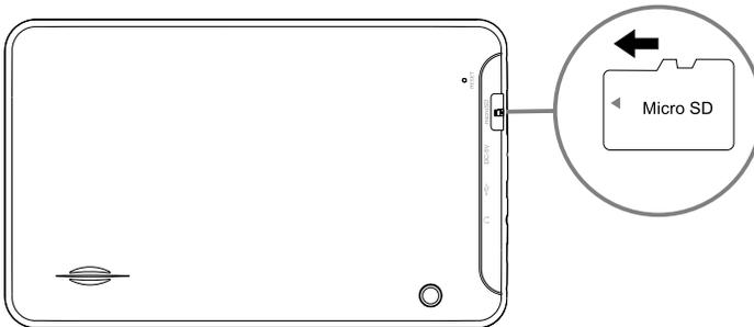
When you want to remove the Micro SD card, touch the SD Card icon in the Notification bar, and select and touch “sdcard is mounted”, then press the card in the slot and it will pop up, take it out gently.
