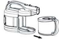
2. Press the dust cup trap door release button to empty the dirt into a trash can.
