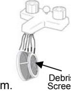
7. To re-assemble the HEPA filter assembly, first insert the HEPA filter onto the dust cup cover making sure to push it all the way in. Then insert the debris screen again making sure that it is pushed all the way up against the dust cup cover.
