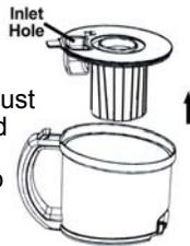
4. When the HEPA Filter assembly is removed from the dust cup, pull off the debris screen first. Then to remove the HEPA Filter from the Dust Cup Cover, hold the HEPA filter with one hand and with the other hand pull the dust cup cover up.
