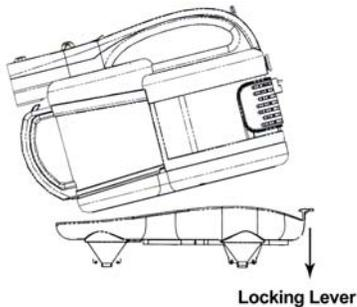
To replace the Mini Canister back onto the caddy, slip the front part of the unit onto the front locking tab of the caddy (see below) and then lock the unit in place by pushing it down until the locking lever clicks in place.
