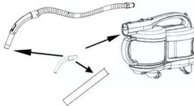
Please note that the crevice tool will only go in the suction hole of the mini canister one way. See illustration below. There is a detent on the top of the crevice tool that locks in place when inserted into the suction hole. To remove the crevice tool from the unit, press the hose release button to allow you to remove the accessory.
