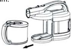
2. You have the option of using the Mini Canister Vacuum as a hand held vacuum or as a canister. To remove the caddy from the main unit, press down on the locking lever and lift the unit up.
