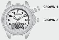
Turn CROWN 1 to cycle through TIME, COMPASS, FORMAT, and DATE. Press CROWN 2 to illuminate watch face (INDIGLO® night-light).
