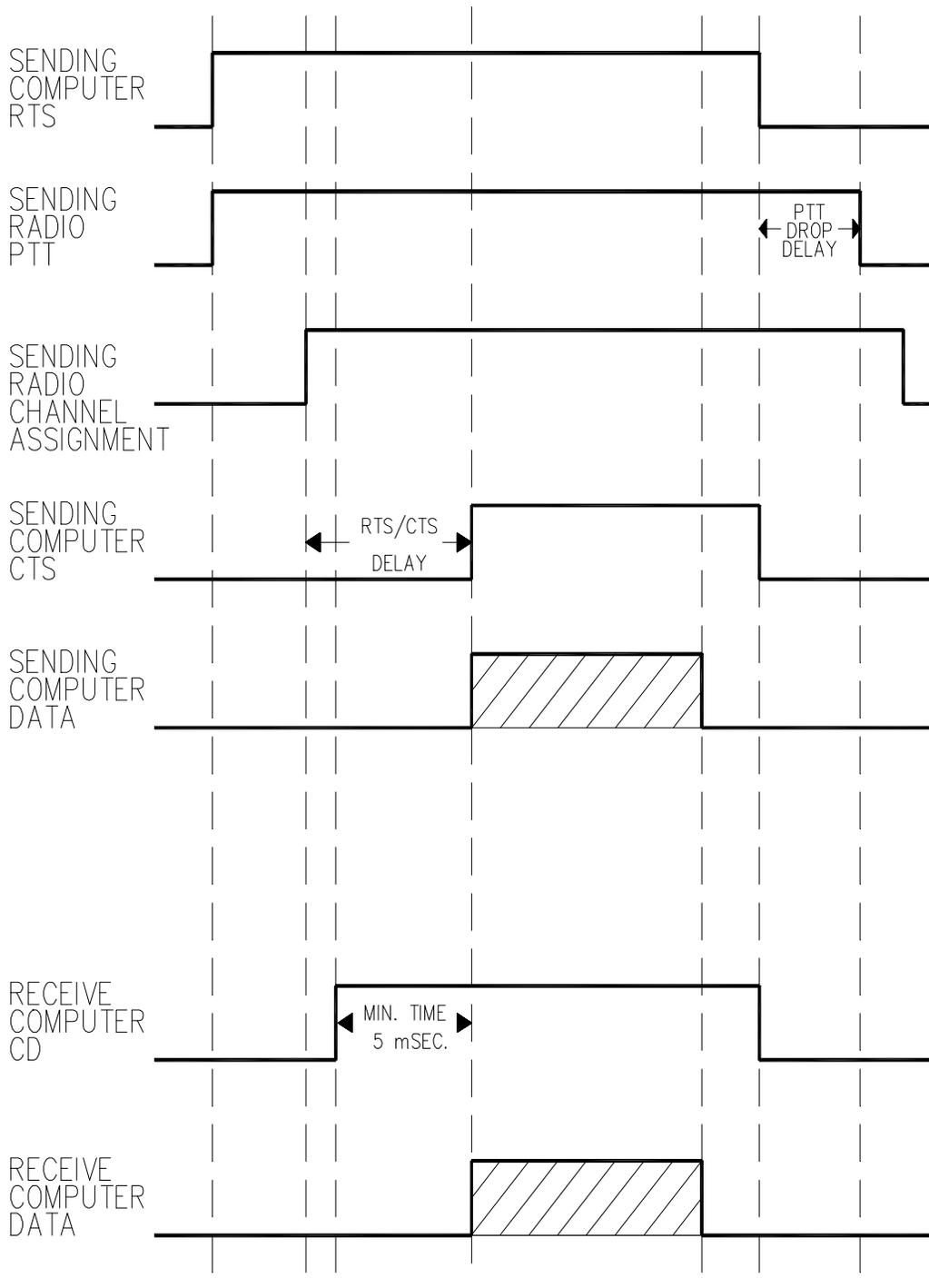
FIGURE 2 MODEM TIMING FOR A GE MARC V TRUNKING SYSTEM USING RTS/CTS HANDSHAKING
