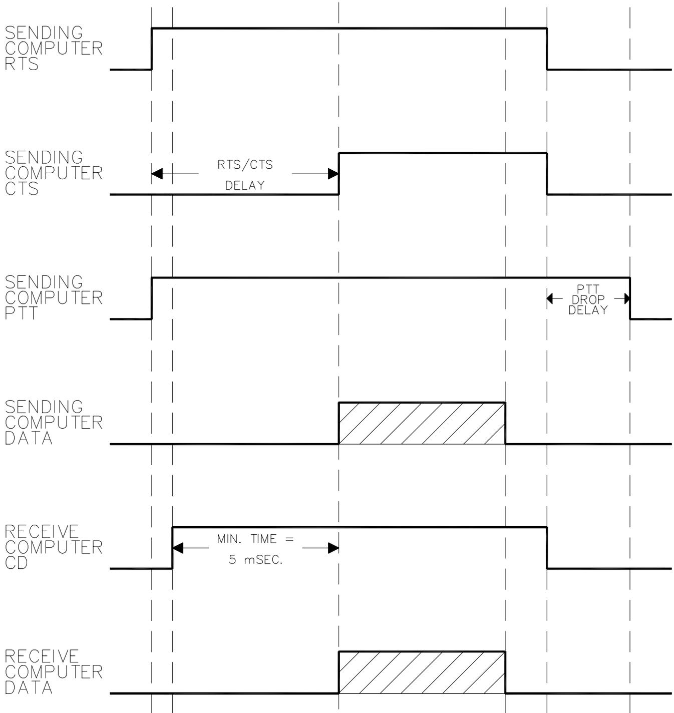
FIGURE 1 MODEM TIMING USING RTS AND CTS
