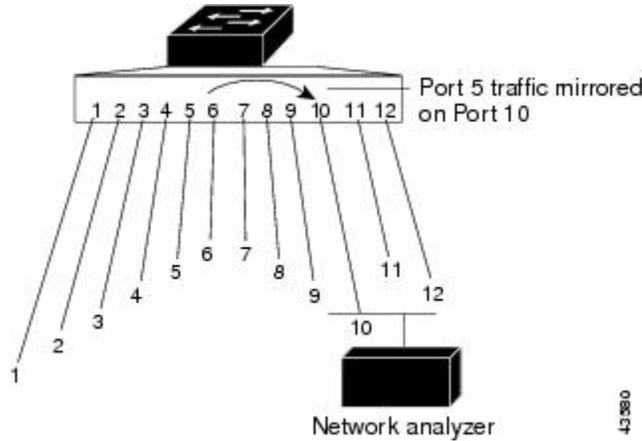
This is an example of a local SPAN in a switch stack, where the source and destination ports reside on different stack members.
