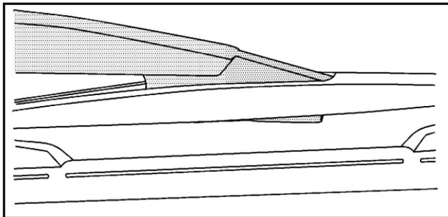
2. Pull the wiper blade assembly away from the backglass. The backglass wiper blade will not lock in a vertical position, so care should be used when pulling it away from the vehicle.
