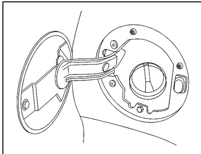
The tethered fuel cap is located behind a hinged fuel door on the driver side of the vehicle. If the vehicle has E85 fuel capability, the fuel cap will be yellow and state that E85 or gasoline can be used. See *Fuel E85 (85% Ethanol)* on page 6-9.
