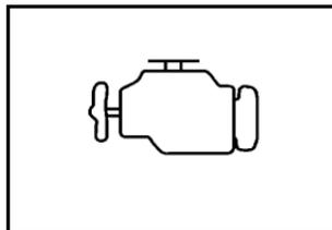
This light should come on when the ignition is on, but the engine is not running, as a check to show it is working. If it does not, have the vehicle serviced by your dealer.
