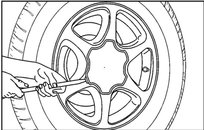
2. If your vehicle has a center cap that covers the wheel fasteners, place the chisel end of the wheel wrench in the slot on the wheel and gently pry the cap out.
