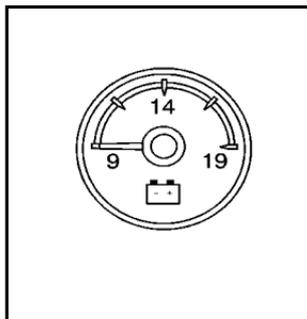
When the engine is not running, but the ignition is on, this gauge shows the battery's state of charge in DC volts.
