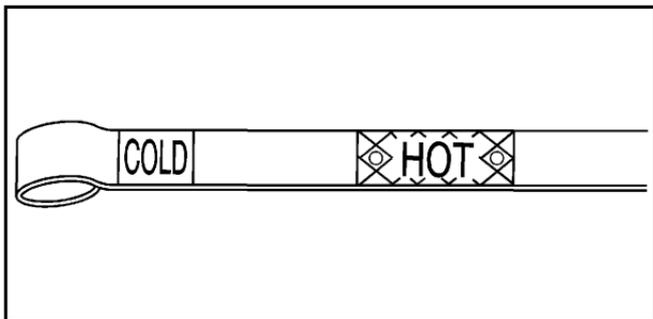
5. If the fluid level is below the COLD check band, add only enough fluid as necessary to bring the level into the COLD band. It does not take much fluid, generally less than 0.5 Liter (1 Pint). Do not overfill.
