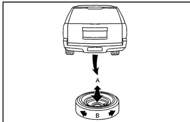
7. Make sure the tire is stored securely. Push, pull (A), and then try to turn (B) the tire. If the tire moves, use the wheel wrench to tighten the cable.
