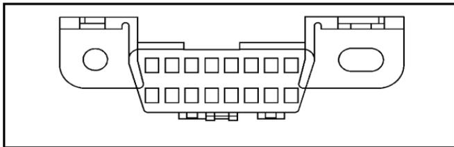
The DLC is under the instrument panel to the left of the steering wheel. See your dealer if assistance is needed.
