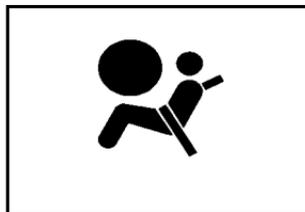
The airbag readiness light comes on solid for a few seconds when the engine is started. If the light does not come on then, have it fixed immediately.
