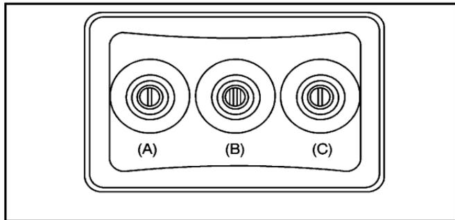
The A/V jacks, located on the rear of the floor console, allow audio or video signals to be connected from an auxiliary device such as a camcorder or a video game unit to the RSE system. Adapter connectors or cables (not included) might be required to connect the auxiliary device to the A/V jacks. Refer to the manufacturer's instructions for proper usage.
