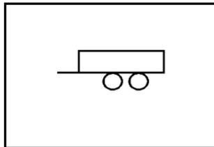
For vehicles with the tow/haul mode feature, this light comes on when the Tow/Haul mode has been activated.
