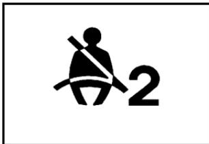
This chime and light sequence is repeated if the passenger remains unbuckled and the vehicle is in motion.
