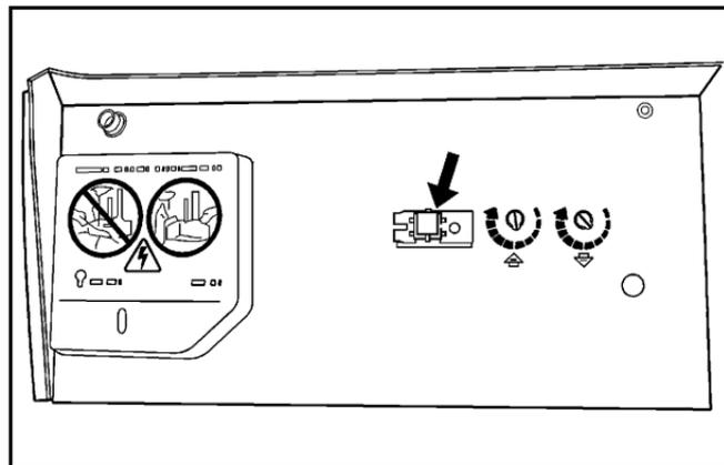
2. Locate in the garage, the garage door opener receiver (motor-head unit). Locate the "Learn" or "Smart" button. It can usually be found where the hanging antenna wire is attached to the motor-head unit and may be a colored button. Press this button. After pressing this button, complete the following steps in less than 30 seconds.
