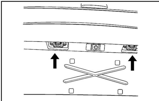
1. Remove the two screws holding each of the license plate lamps to the molding that is part of the liftgate.
