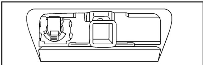
The vehicle is equipped with the seven-wire trailer towing harness. This harness with a seven-pin universal trailer connector is attached to a bracket on the hitch platform.
