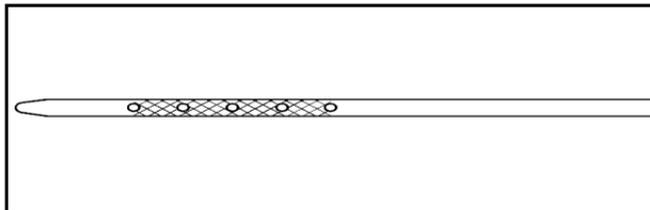
If the oil is below the cross-hatched area at the tip of the dipstick, add at least one quart/liter of the recommended oil. This section explains what kind of oil to use. For engine oil crankcase capacity, see *Capacities and Specifications on page 6-126*.
