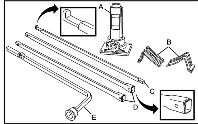
2. Remove the wing nut (B) used to retain the tool bag by turning it counterclockwise.
