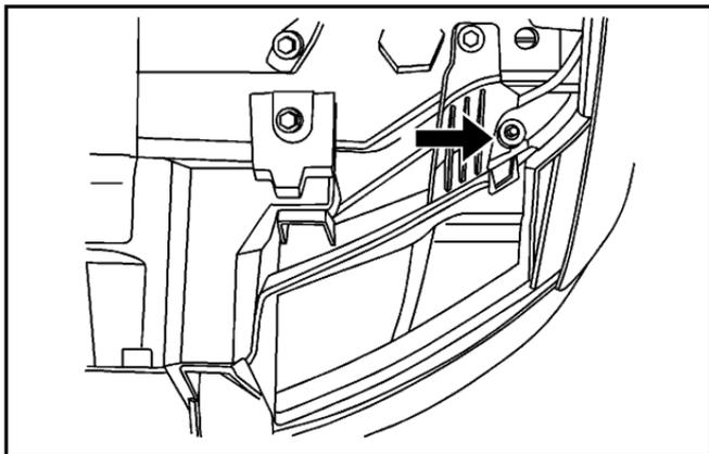
7. Locate the vertical headlamp aiming screws, which are under the hood near each headlamp assembly. The adjustment screw can be turned with an E8 Torx<sup>®</sup> socket.
