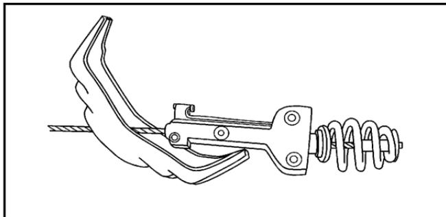
2. Tilt the tire toward the vehicle. Separate the tire/wheel retainer (G) from the guide pin. Pull the pin through the center of the wheel. Tilt the retainer down through the center wheel opening.
