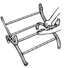
3 Hook one end of rod over small indentation at end of cross brace (A).
