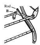
5 With casters on floor, insert ends of Cradle Support Rod through holes in top of curved leg section. **NOTE:** Curved edge of Cradle Support Rod <u>must</u> be angled outward as shown.
