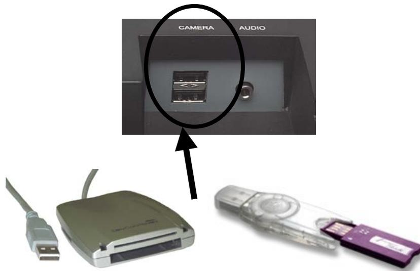
**Figure 15 – Connecting a Card-Reader or Thumb-drive**
