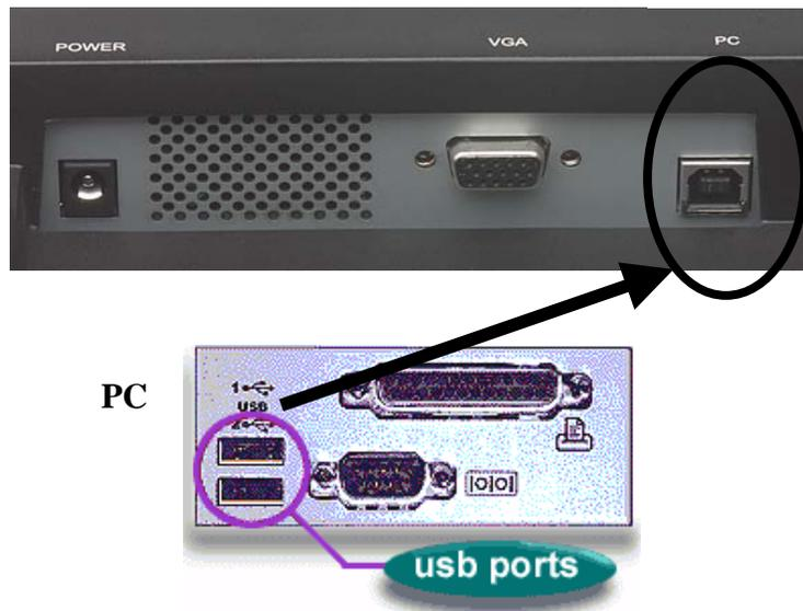
**Figure 7 – Connecting a PC to MemoryFrame**
