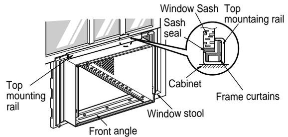
**NOTE:** Do not shut the window so tightly that movement of the frame curtains is restricted.
