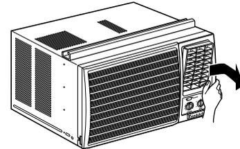
Step 4. Lift the inlet grille and secure the front grille with a type A screw. Lower the inlet grille into place.
