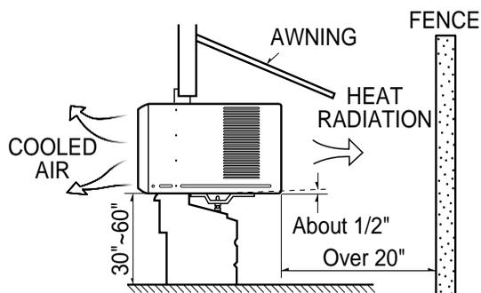
**CAUTION:** All side louvers of the cabinet must remain exposed to the outside of the structure.
