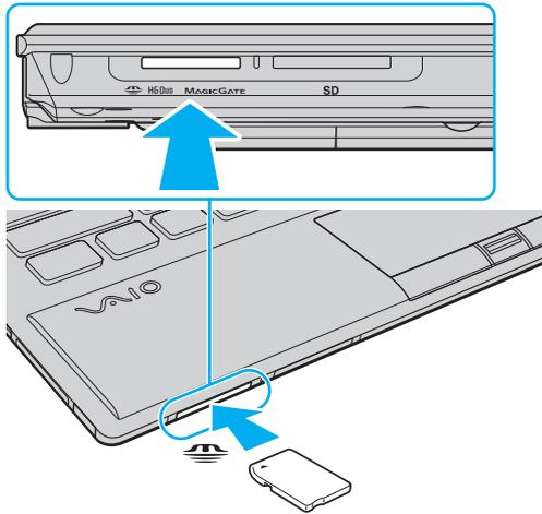
**!** Before using "Memory Stick Micro" ("M2"), be sure to insert it into an "M2" Duo adaptor. If you insert the media directly into the "Memory Stick Duo" slot without the adaptor, you may not be able to remove it from the slot.
