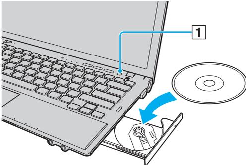
**!** Do not exert pressure on the drive tray. Be sure to hold the bottom of the drive tray when placing/removing a disc onto/from the tray.
