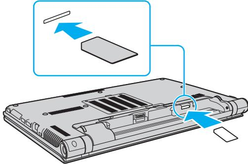
! Do not touch the printed circuit on the SIM card. Be sure to hold your computer firmly before inserting or removing the card.
