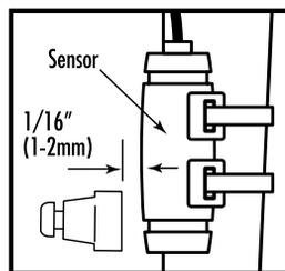
1. Position the axiom unit to the inside of either the right or left fork blade anywhere from 3-6 inches up from the fork blade tip. Attach the axiom to the fork blade with the quick ties but do not tighten the ties completely until final adjustment is complete.
