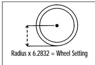
Measure wheel radius (including tire) in mm and multiply by 6.2832=Wheel setting number.
