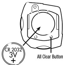
1. Remove the battery cover from the back side of the computer using a narrow flat blade screwdriver.
