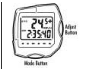
The Axiom is equipped with 2 buttons that control the function of the unit.
