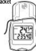
The Fisher Axiom Computer attaches to the mounting bracket by sliding the unit onto the bracket from the back until it snaps firmly into position. To remove the computer from the bracket, place your thumb against the back of the mounting bracket and pull the computer toward you with your index finger.
