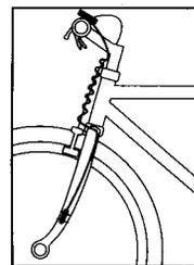
1. Route the axiom wire up the back of the fork blade or wind the wire around the blade, making sure that the wire is not loose and that you leave enough wire to reach the handlebar. Secure the wire to the fork blade immediately above the axiom and at the top of the fork blade, using the adhesive strips that are provided or electrical tape.
