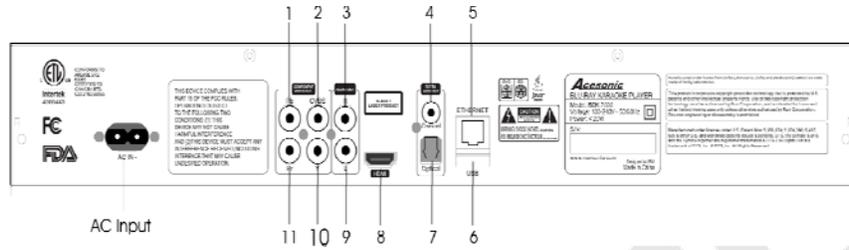
**AC Cord Input** - Connection to the auto-detect AC power supply (100-240V,50-60 Hz).
