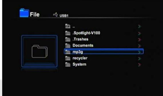
Individual files can be selected using the **Direction Buttons** [▲/▼] and pressing the **ENTER** Button or **Play Button** to play it. Compatible file types are: MP3, WAV, WMA, MPEG-1, MPEG-2 (MPG/VOB), MPEG-4 (AVI), JPEG, and MP3G.
