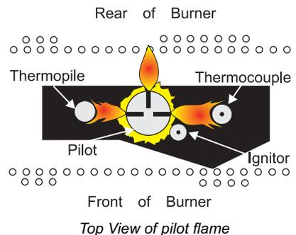
Incorrect flame pattern will have small, probably yellow flames, not coming into proper contact with the rear of the burner or thermopile.
