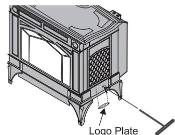
To adjust the aeration: use the allen key to turn the turning gear which will adjust the air shutter. Open the air shutter for a blue flame or close it for a more yellow flame. This adjustment is performed by a qualified installer. The factory setting should be sufficient for most installations.
