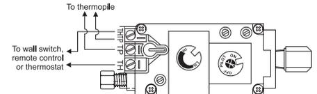
box (protection from extreme heat is very important). Run wires from the fireplace to that location, use Thermostat Wire Table.
