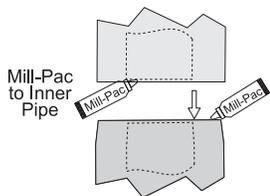
Hint: Apply the sealant (Mill-Pac and/or high temperature silicone) to the outer pipe before connecting the inner pipe.
