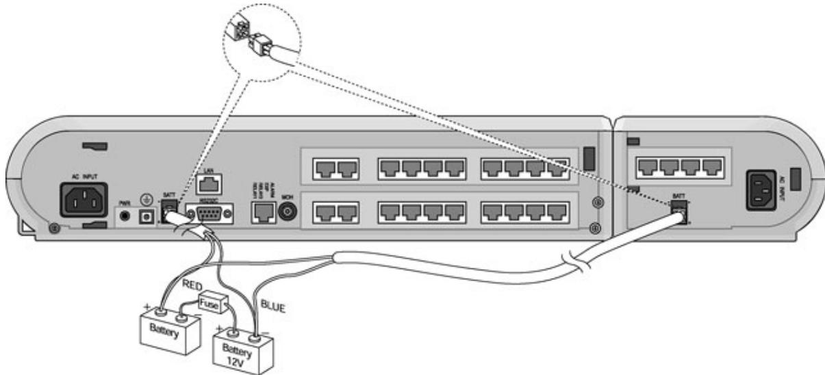
**Figure 4.4 External Back Up Battery Installation**
