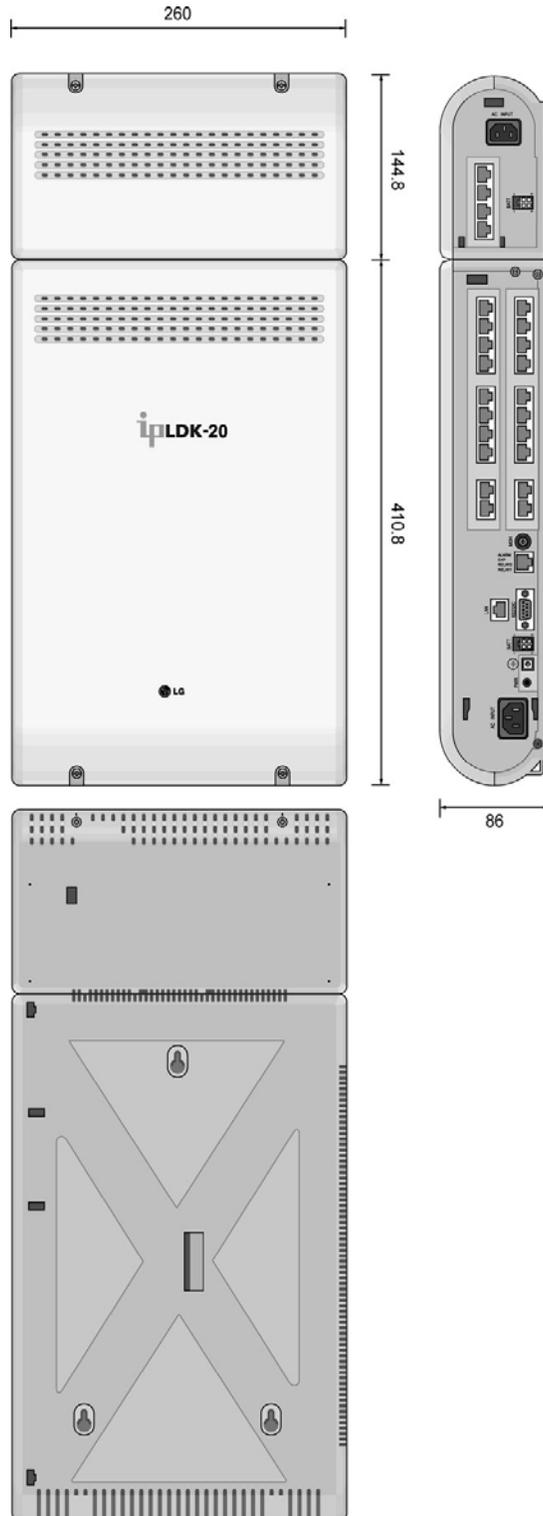
Figure 2.2.3 KSU with expansion module exterior and dimension
