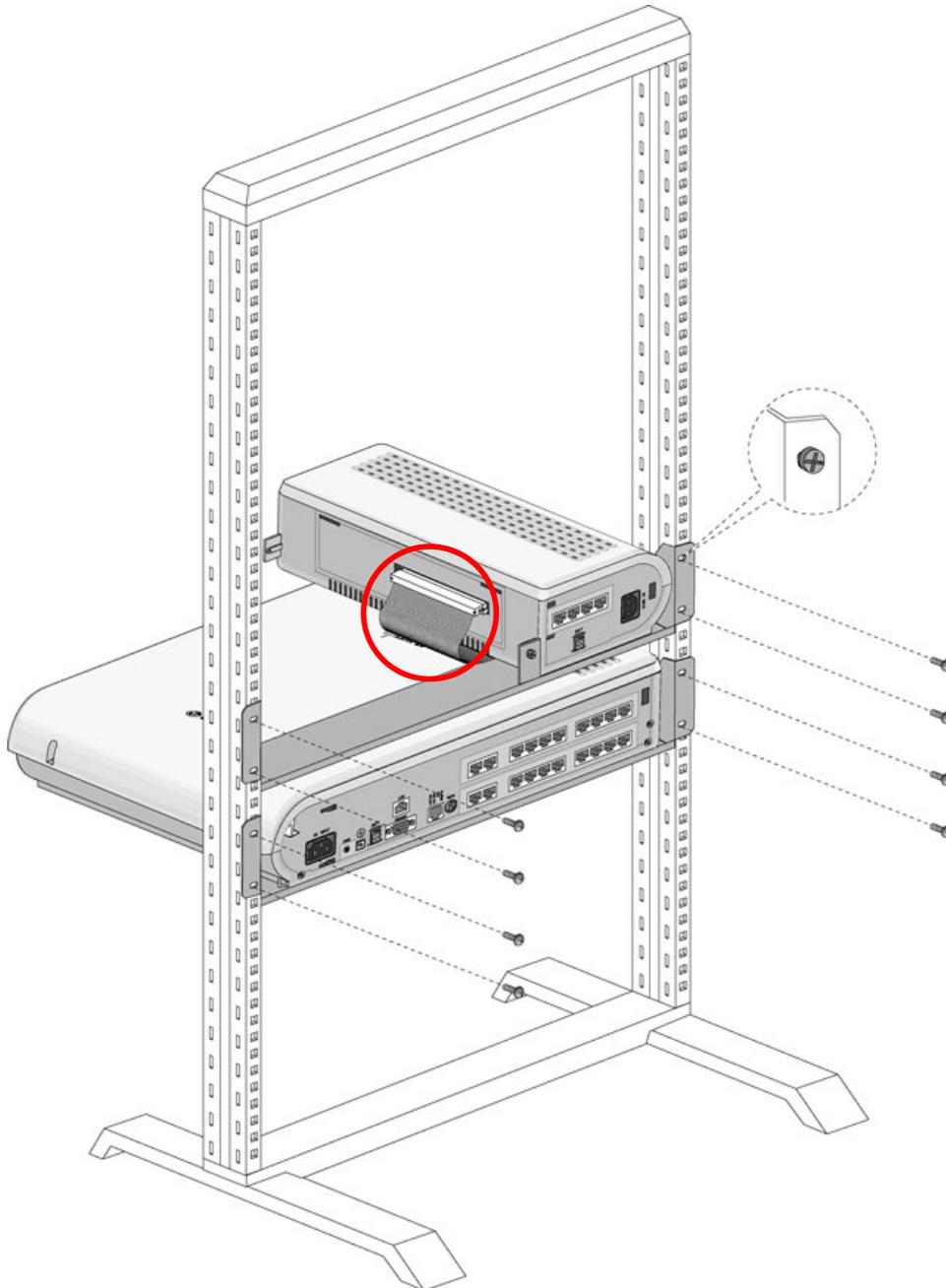
Figure 4.3.3.4 Module Rack Mounting
