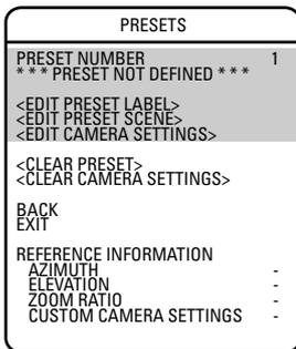
The Spectra III SE dome system has 80 programmable preset positions. Each preset can be programmed to use pan, tilt, and all programmable camera settings.
