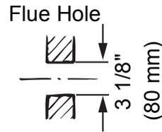
**NOTICE** Use a template (included) to determine allowable location of the flue hole.
