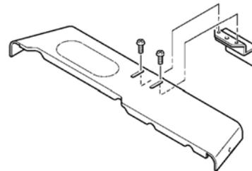
6. Install the wall bracket with two screws. Install the top spacer by clipping the spacer into the wall brackets and attaching it to the heater with 2 screws.
