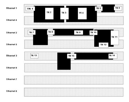
If Ethernet 1 is in use, any networks that overlap Ethernet 1 (meaning that they share the same backplane resources) are unavailable. As the diagram shows, using Ethernet 1 makes TR 1 through 6 unavailable.
