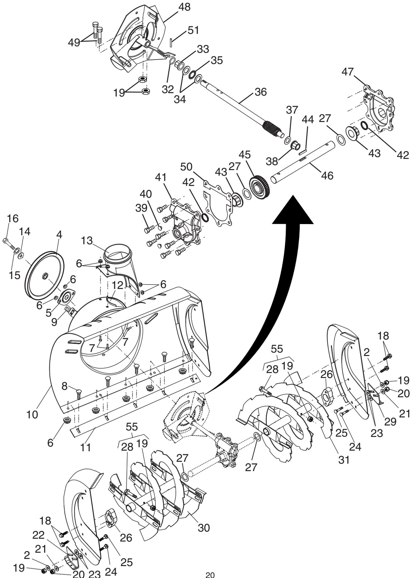
**REPAIR PARTS****AUGER HOUSING / IMPELLER ASSEMBLY****SNOW THROWER - - MODEL NO. 8527STE (HL8527STEA), PRODUCT NO. 954 22 36-54**
